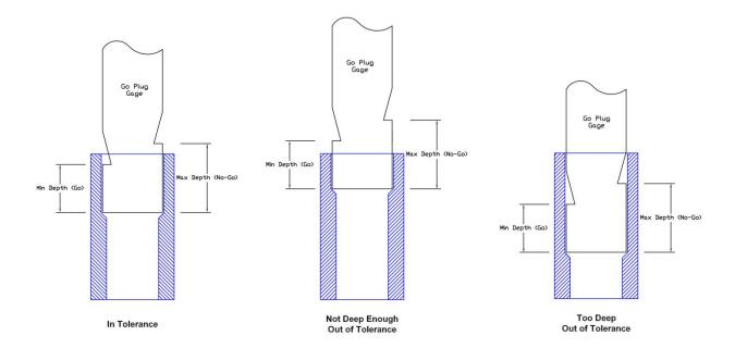
Angular transitions between two internal diameters can be a challenge to measure, (see the above illustration). The chamfer or radius on the end of the plug gage that enters the hole needs to be as small as possible. If they are too large, the radius or chamfer will allow the gage to seat on the transition angle between the two holes.
