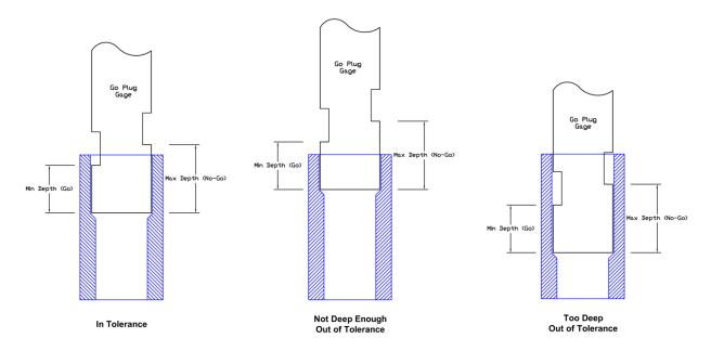
Square or flatted notches have a square or rectangular flat plunged into the diameter at a specific depth (see illustration above). They function the same, as the "whistle" notch. The bottom of the notch is the gage plane used to measure the depth of the hole. This design can be confusing. Some users question if the top of the square or flatted notch is also a measuring plane. Although it is done in some rare instances, most will use the bottom of the flatted notch as the gage plane.
