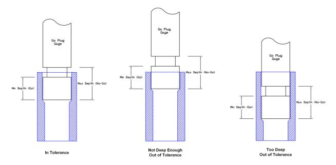
Depth grooves function as depth inspection tools as well (see illustration above). These also have advantages and limitations. In the case of the depth groove, the bottom of the groove acts as the minimum (Go) depth and the top of the groove represents the maximum (No-Go) depth. The nice thing is that you have a groove that goes around the circumference of the gage. The user does not need to rotate the gage in the hole to see the notch as you would with a
